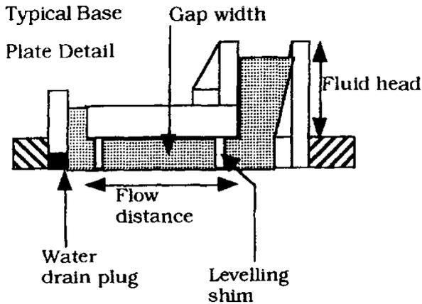
Pouring should be from one side of the void to eliminate any air or presoaking water from being trapped under the baseplate.
